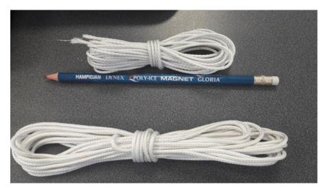
**Figure 1:** Prototype Hampidjan dyneema braided lead core weighted line of 10 g/m. Note that any commercial product needs to be very low visibility so as not to affect fishing efficacy.
